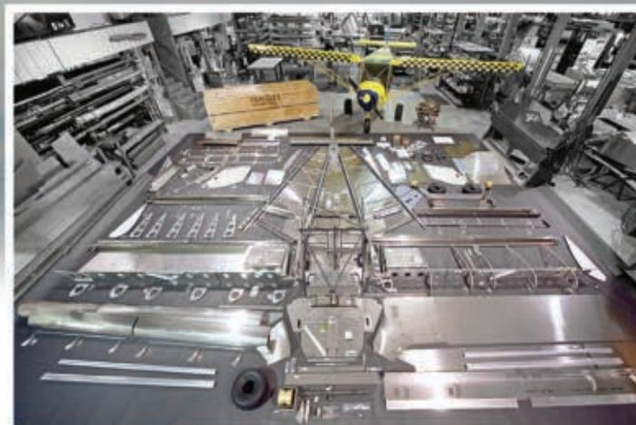
**The Complete Kit with extensive CNC-cut match-drilled parts.**
